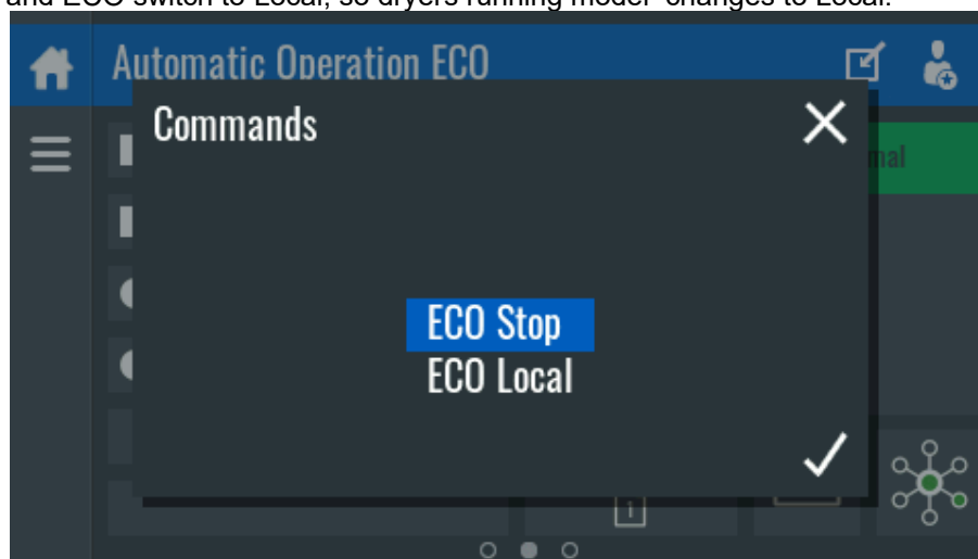
Figure: ECO switch to Local
