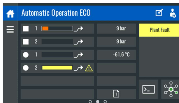
Figure 20 Plant fault (HTM standard)
