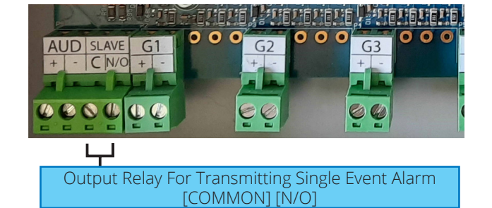
Figure 17 - Output alarm relay signal connection.
