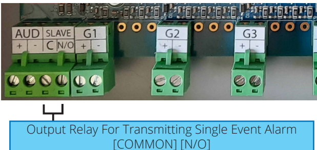
Figure 17 - Output alarm relay signal connection.
