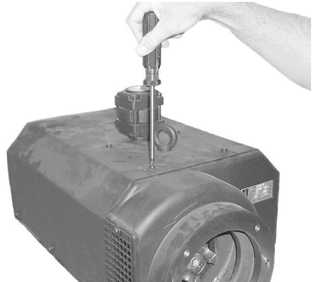
Fig. 3 - Removing the Access Panel
