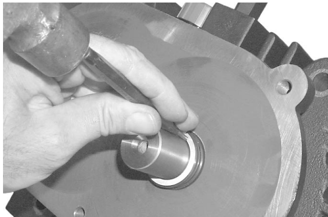
Fig. 26 - Installing the Labyrinth/Seal Sleeve
