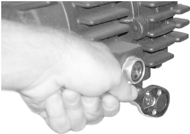
Fig. 4 - Draining the Oil
