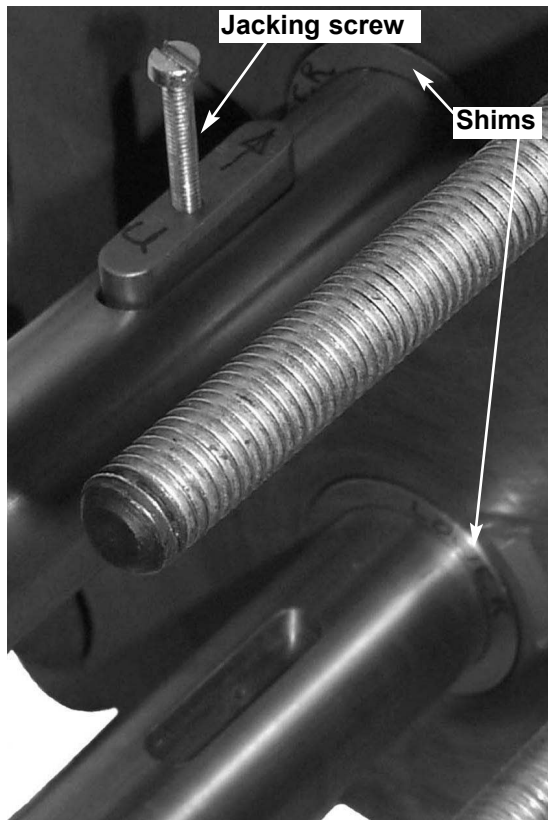
Fig. 14 - Removing Shaft Keys and Shims
