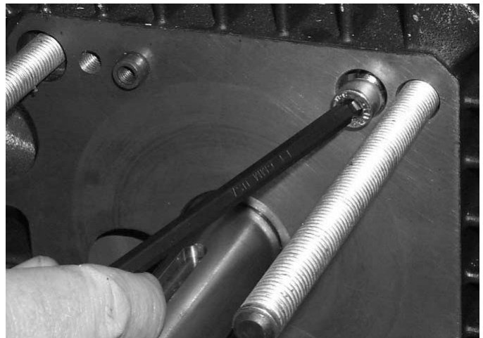
Fig. 16 - Removing the "A-side" Endplate
