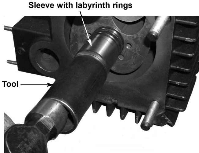
Fig. 30 - Installing the B-side Shaft Seal Sleeve
