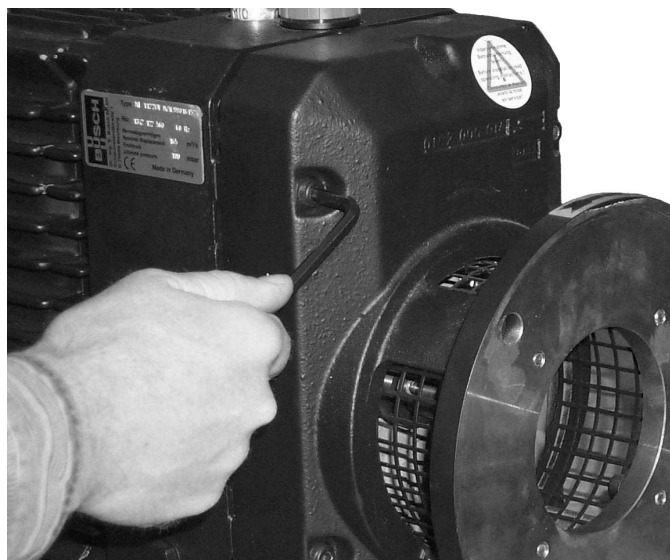
Fig 6 - Removing the Motor Mounting Bracket
