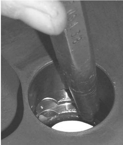
Fig. 21 - Removing the Shaft Seal Cartridge Assembly
