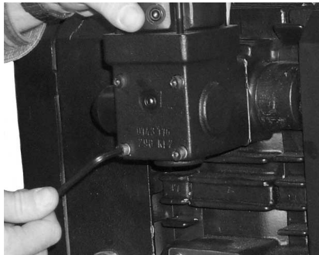
Fig 5 - Removing the Inlet Flange Assembly
