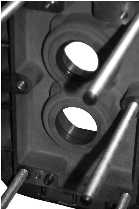
Fig. 23 - Removing the "A-side" Endplate Seals
