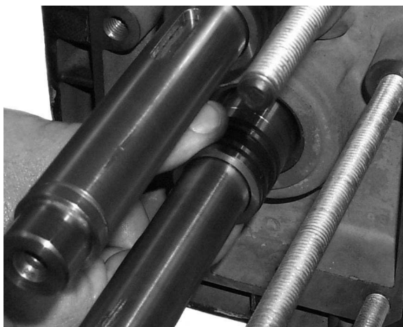
Fig. 27 - Installing "A-side" Shaft Seal Sleeves
