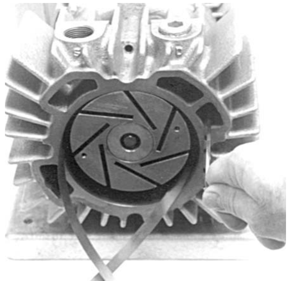
Fig. 16 - Setting the Radial Clearance
