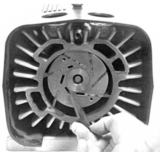
Fig. 8 - Inspecting the Vanes
