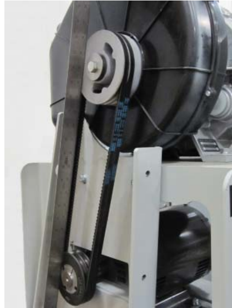
Figure 6.2 Belt Alignment - Straight Edge
