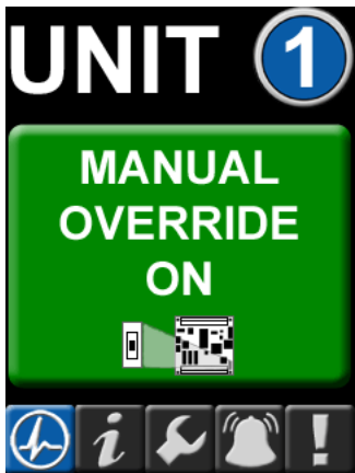
3.5" Unit screen with Manual Override selected
