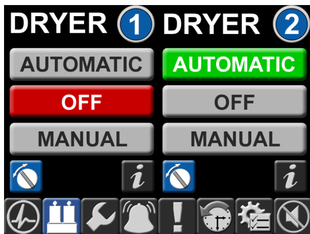
Dryer 2 is in Automatic mode, Dryer 1 is in Off position
