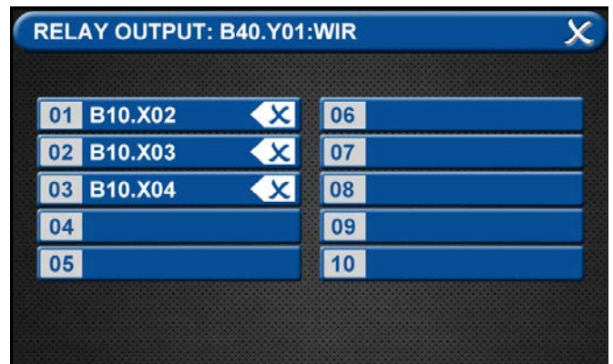
Figure 160: Relay Output Many Signals
